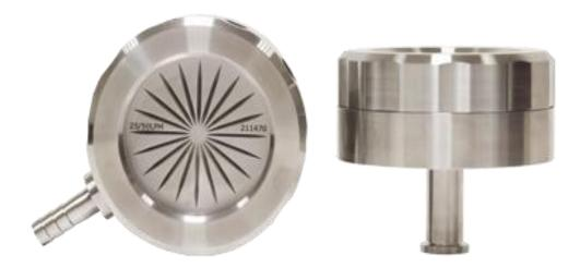
The slit is approximately of length of the petridish. The petridish is rotated at a particular speed under the slit. One complete turn is made during the sampling operation.
